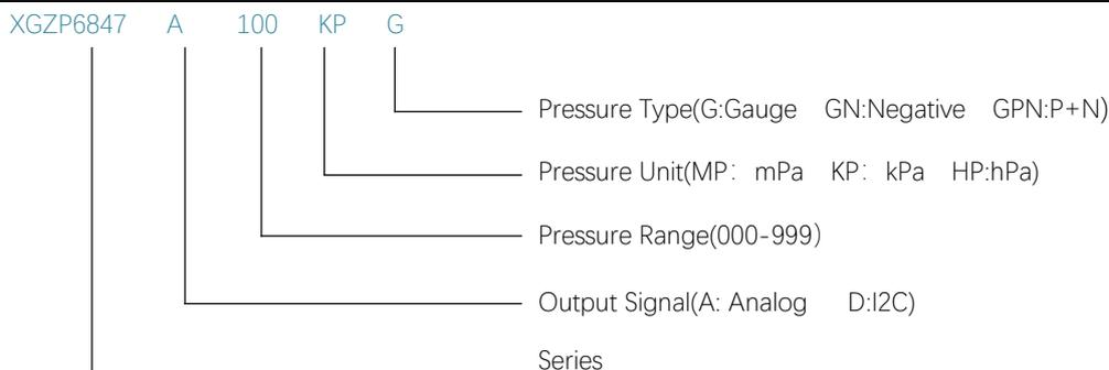
Note: 1. Voltage 5Vdc as default value, add 33(or 30) behind model signify 3.3V(or 3.0V) power supply, e.g. : XGZP6847A040KPG33.
